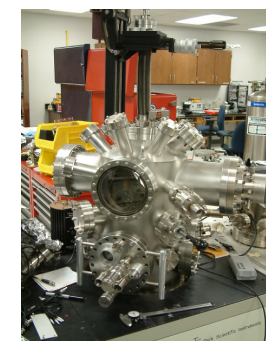
Picture of 2 nd STM chamber at LSU where Ag and Ti deposition will occur.
