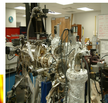
Picture of an STM chamber at LSU where Ag and Ti deposition do occur.
